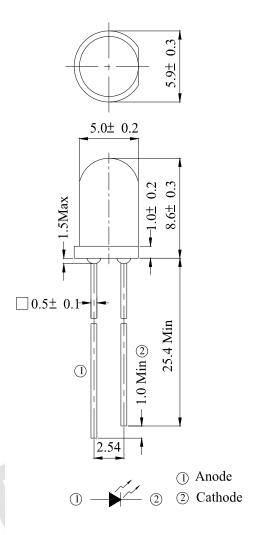
Note: Tolerances unless dimensions ±0.25mm
